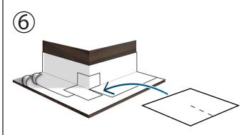
Cut two 8"x8" patches and install on the outside corner to provide reinforcement.
