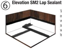
Tool sealant over all membrane edges, including those on the vertical walls and the horizontal surface. Sealant is applied to all waterproofing membrane termination points.
