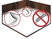
Install Elevation S60 36" covering the deck and running a min. 3" up the vertical wall. At all inside corners stick excess vertical S60 36" membrane to itself and fold over to one side of the corner, thus eliminating cuts or terminations in the membrane. Ensure S60 36" fits tight into the corner. wall.
