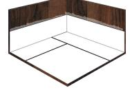
Install Elevation S60 12" 8 to 9 inches up the vertical wall, running down the wall and on to the horizontal deck a minimum of 3", overlap creates a positive shingle effect.
