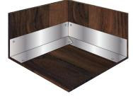
Bend vertical leg to match contour of the corner, while bending vertical leg properly lap horizontal leg to fit the corner. Fasten flashing in place.
