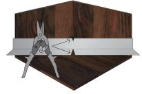
Before installing base flashing at inside corner, make a cut on the horizontal leg at corner's turn (approx 30 degrees to allow overlap after folding) and relief cut at top to prevent puckering in corner
